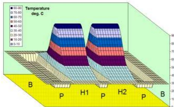
Figure 5 – Temperature field of the integral structure (see Figure 1b) without the impact of the heat transfer across the flow
